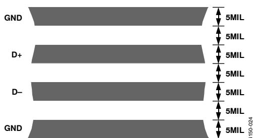
Figure 24. Typical Arrangement of Signal Tracks
